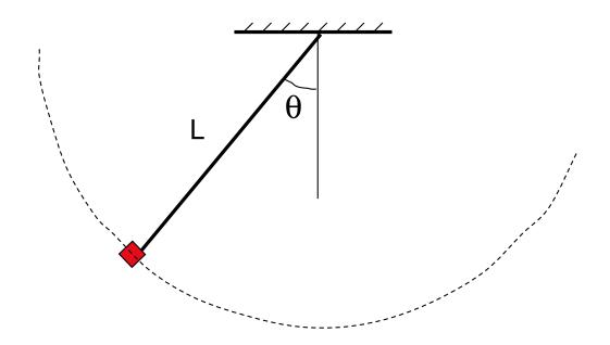
This is a bit tricky. As the bob is passing through the bottom of the arc, gravity and tension will both be in the vertical, and they will have to accommodate centripetal acceleration. The f.b.d. looks like and N.S.L. becomes:
