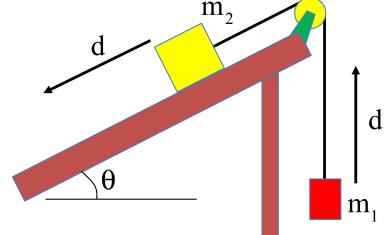
We'll assume the block accelerates *down* the incline. So what's its velocity once it has traveled a distance *d* units down the incline?
